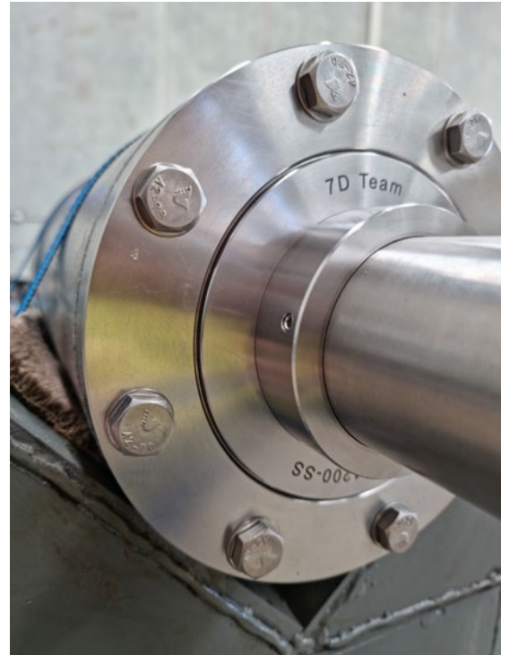
Bulwark Bearing Guard on a 7D Team bearing assembly
